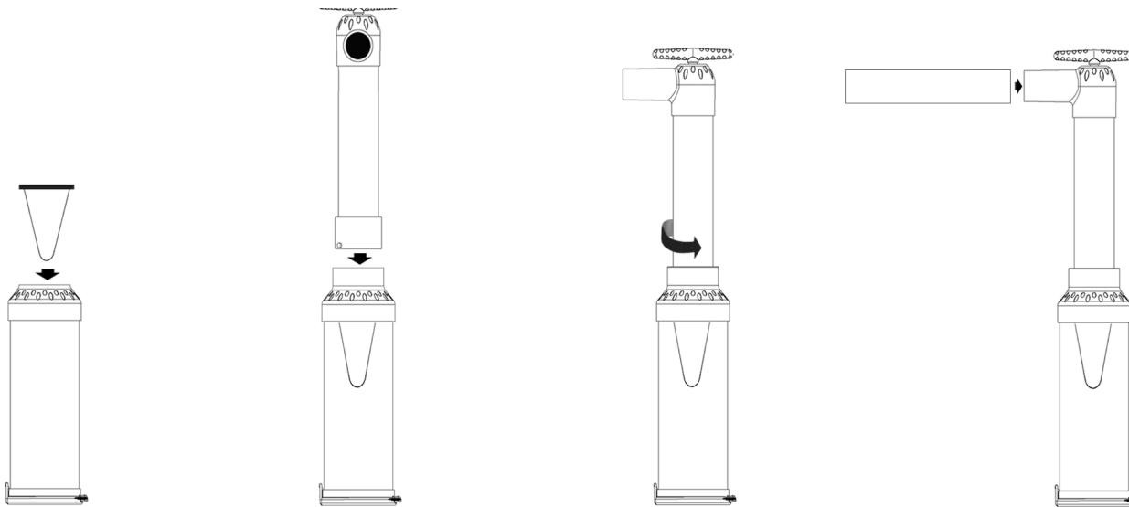
Place the filter cone into the top of the debris chamber.
