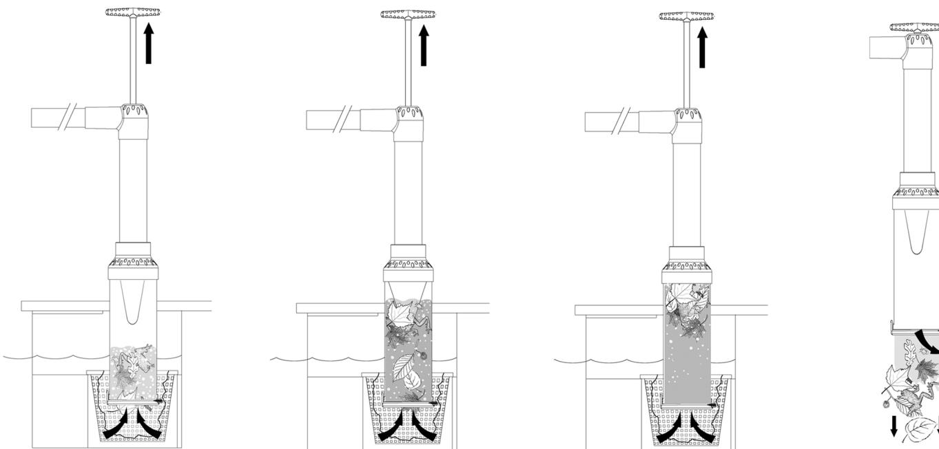
Place the Skimmer Basket Vac™ into the skimmer basket. To start, hold the unit **above the bottom of the basket** and pull the Pump Handle up.
