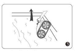
You should take the cleaner out vertically to drain inside water out quickly.
