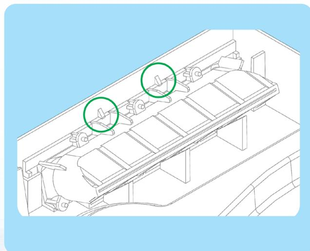
4. Press until triangular tabs snap back over valve mounts.
