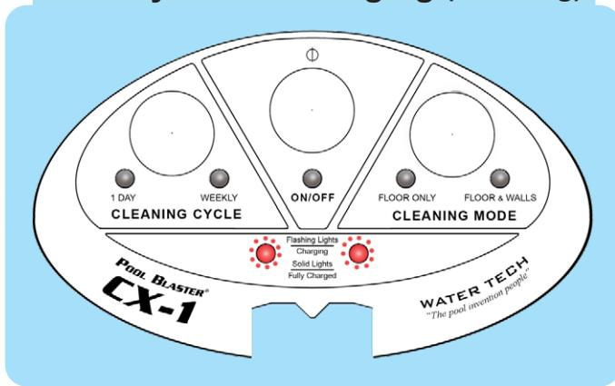
As both battery packs are charging, the LEDs (shown above) will flash.
