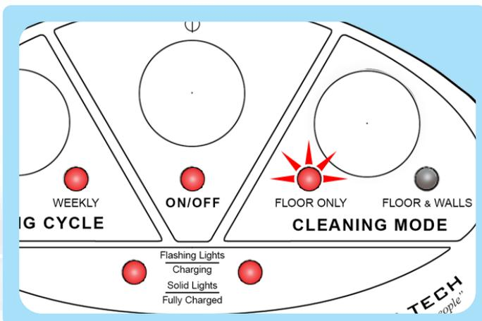
4. Wait for the “Floor Only” LED to stop flashing, then press the “Cleaning Mode” button one time.
