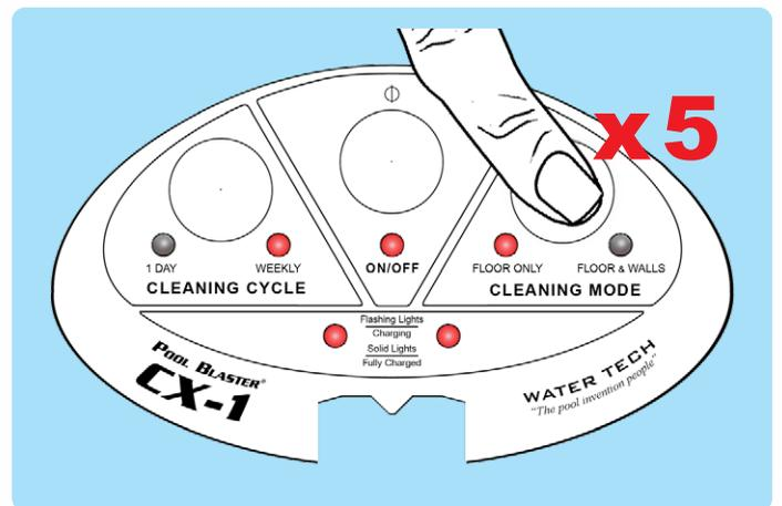
3. The “Floor Only” LED light will flash rapidly to indicate proper entry.
