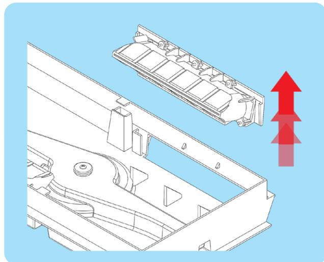
2. While still pressing outward, lift the valve mount up and out of the bottom cover. Rinse out the valve mounts and bottom cover.
