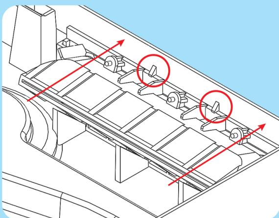
1. Press outward on the bottom cover so the valve mount can fit around triangular tabs (shown circled above).
