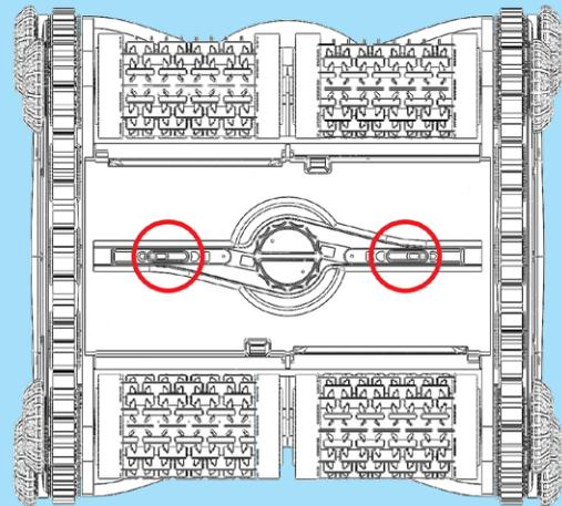
You will feel the knob “snap” as the lock is undone. Note that the locks will move inwards. This means the cover is unlocked.
