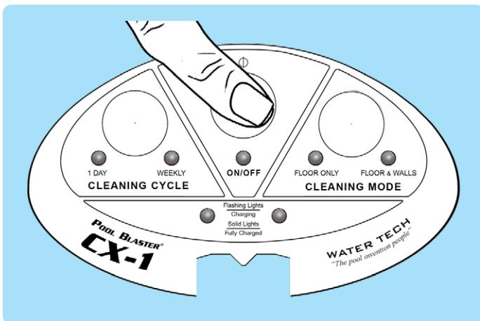
2. Within 5 seconds of turning the robot ON, press the “Cleaning Mode” button 5 times.
