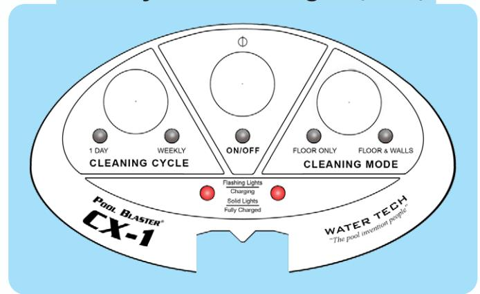
Once a battery pack is fully charged, its LED will turn solid. It is common for 1 LED to turn solid before the other.
