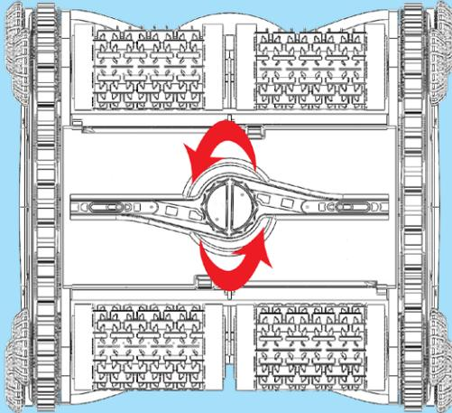
To remove the Filter Bag, flip the CX-1 upside-down and turn the knob on the bottom counter-clockwise.
