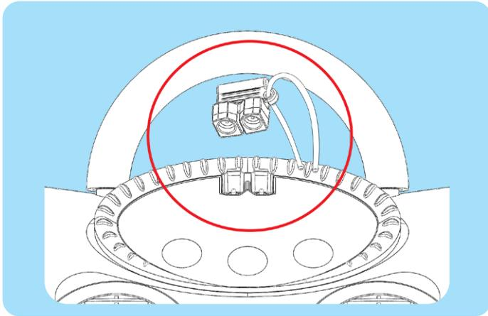
When the CX-1 is done charging, it's important that you **DO NOT** submerge the CX-1 in water without replacing the rubber plug covering the charging jack. Failure to follow this step could damage your unit.
