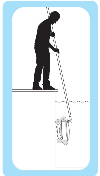
Lift the CX-1 to the surface using a slow, steady pulling motion. Remember, the CX-1 is heavy while full of water.
