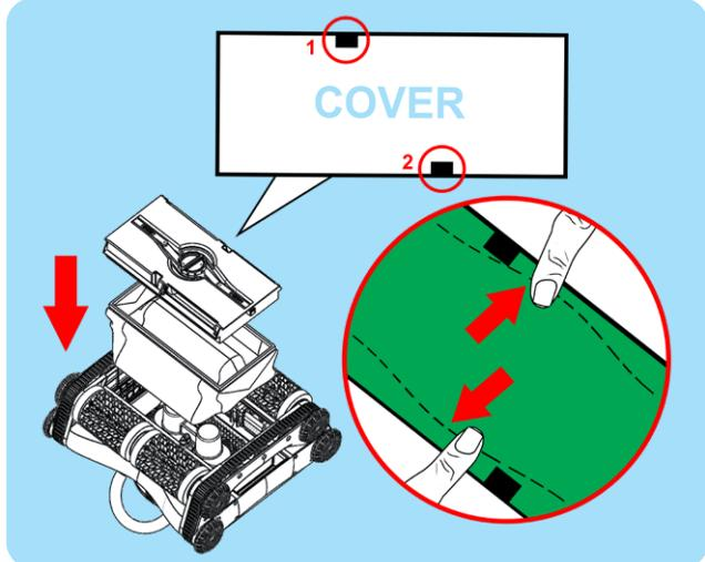
Re-insert the filter bag with the cover on top. Make sure you lock the bag under the two locking tabs (Illustrated above as #1 and #2). Then, insert bag into unit as you lower the cover into place.
